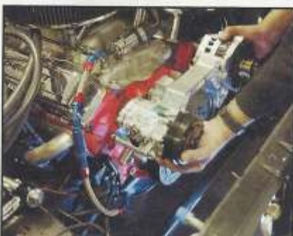
•The FrontRunner accessory mount system includes a new compressor, 140 amp alternator, mounts, brackets and stainless steel hardware for a clean, simple installation.
