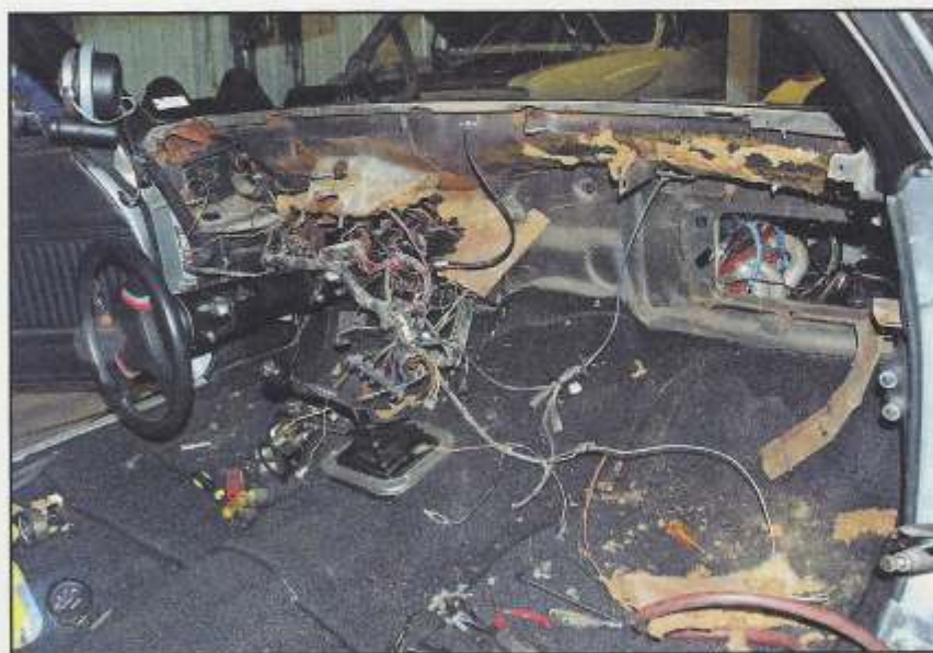
•With the dash and heater assembly out of the way, we now have unimpeded access to the firewall and passenger side kick panel.
