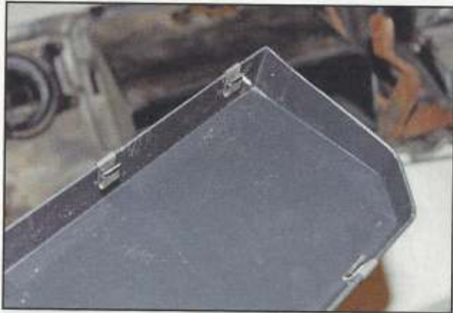
•These S-clips retain the new cap to the box, as it's slid in place on the outside of the cut.
