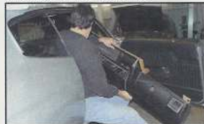
•After removing the front seat, the dash pad was removed next, and then the complete dash assembly. We set it aside for modifications that are covered in a sidebar.
