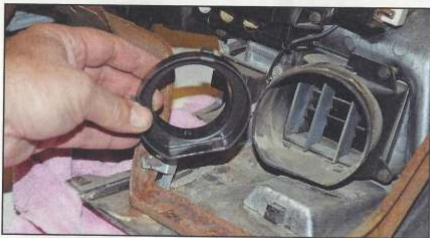
•Hose adapters are also include with the kit, allowing you to retain the dash-mounted vents. The plastic pieces are formed for a perfect fit.
