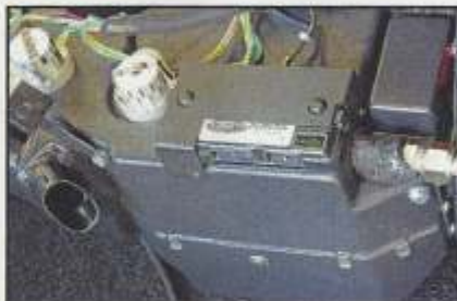
• The Sure Fit kit includes a new heater/evaporator combo unit, and everything else needed to complete the installation. A microprocessor (ECU) mounted on top of the box itself controls all heating and cooling activities by signaling the electronic servos to do your bidding.
