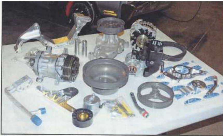
•The FrontRunner accessory mount system includes a new compressor, 140 amp alternator, mounts, brackets and stainless steel hardware for a clean, simple installation.
