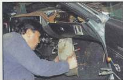
•With the outside heater box removed from the firewall, we directed our attention to the inside where we disconnected all the factory cables and wire connections before removing the inside heater box.
