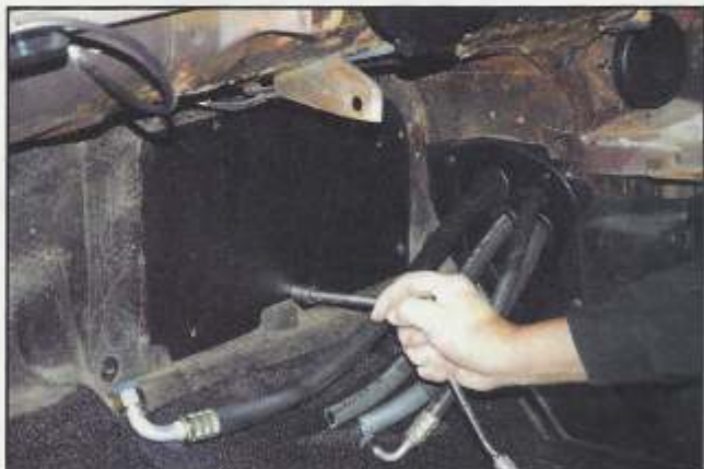
• Once the hoses are routed and the kick panel secured, the metal firewall plate is bolted in place using the mounting holes for the original heater assembly.
