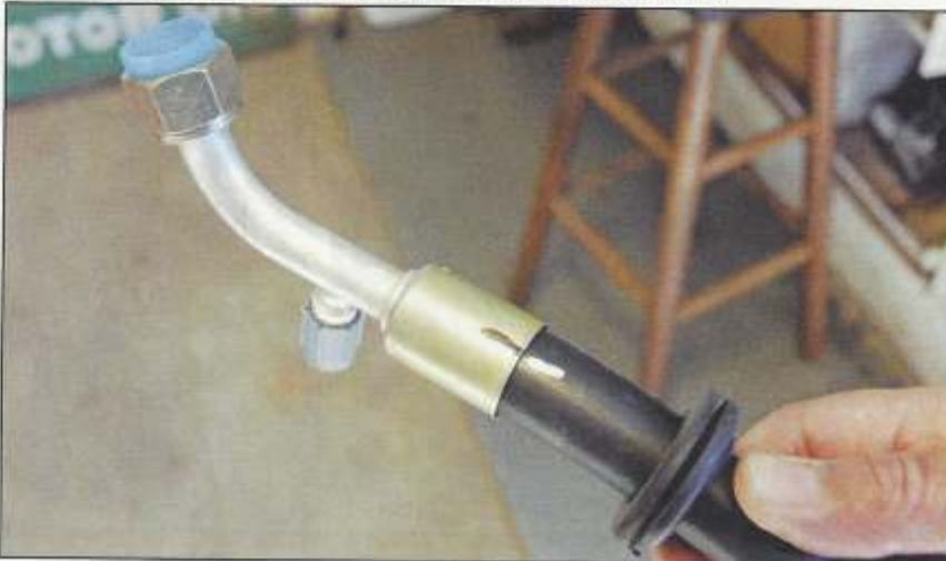
•Before beginning the crimping operation, make sure your marks are lined up to ensure proper clocking of the hose and fitting.
