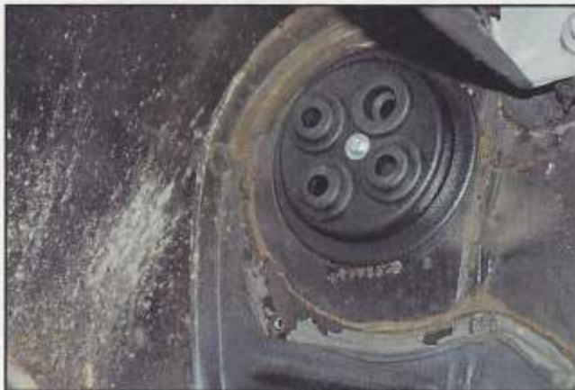
• This block-off plate installs where the original blower fan previously resided, and provides support for the hoses once they are routed through to the engine compartment.
