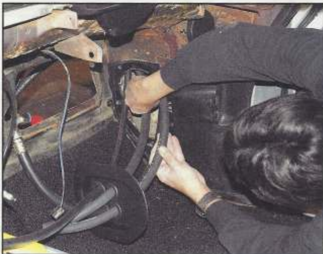
• Once the hoses are routed and the kick panel secured, the metal firewall plate is bolted in place using the mounting holes for the original heater assembly.
