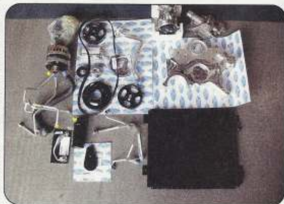
These are all the parts from Vintage Air for under the hood, including all of the Front Runner components, water pump, alternator, power steering pump, air conditioning compressor, lines, condenser and receiver dryer.
