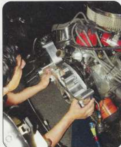
With the crank seal installed and the gaskets between the block and the new timing cover, it is slid into place on the front of the engine.
