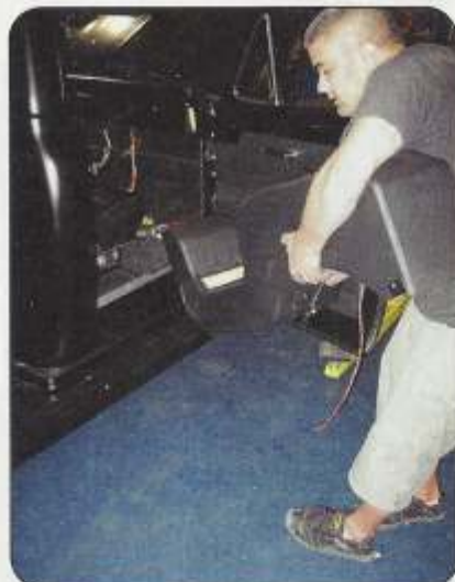
That meant that the center console would have to be removed and set aside until everything was installed and then it could go back in.
