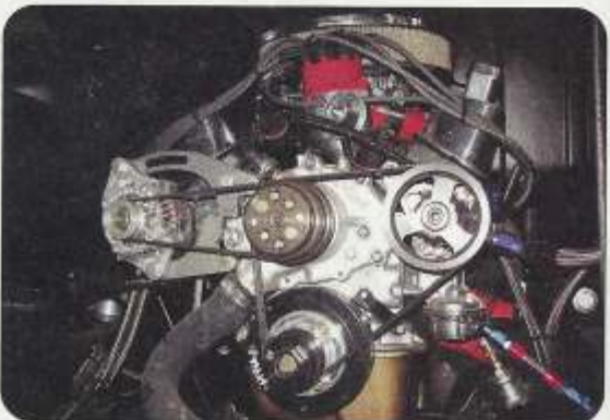
OK, here was issue number one. For a street-driven vehicle this setup wasn't spinning the alternator and the power steering pump fast enough at cruising speed on the freeway. Notice that the grille and radiator were removed to make it easier to clearly see what was going on with the front of the engine.
