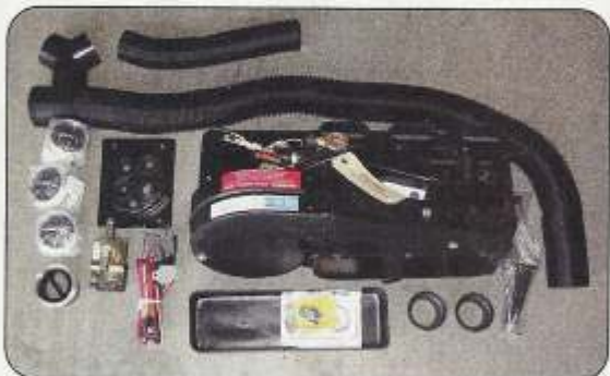
All of these components are the parts from the firewall back and include the bulkhead cover, electronic heater control valve, vents, controller and the big plastic box that houses the heater core, evaporator, expansion valve, blower motor and all of the ducts that direct the air where you tell it to go.
