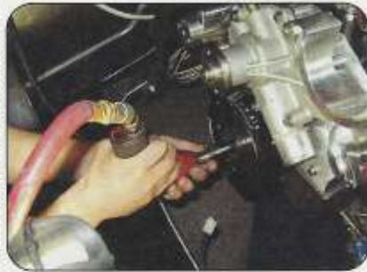
The harmonic balancer is the next item to be reinstalled.
