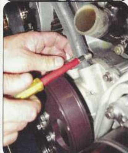
Once everything inside the cab was buttoned up, the heater hoses were run from the bulkhead to the front of the engine.
