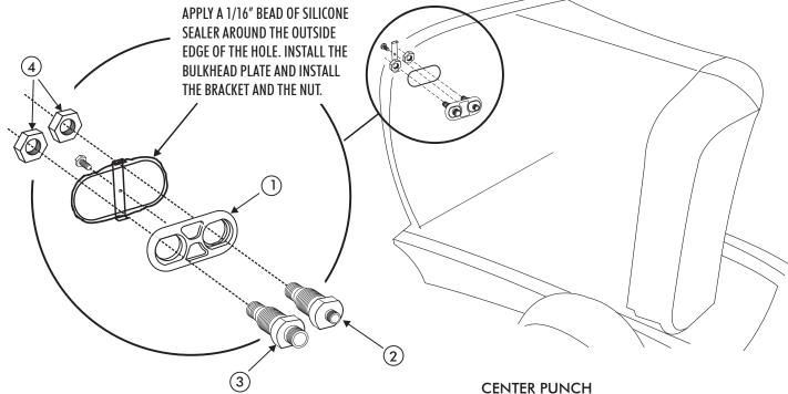
MAKE CIRCULAR ENDS OF OPENING WITH 1-1/4" HOLE SAW. CENTER PUNCH PILOT HOLE BETWEEN CENTERS AS SHOWN. WHEN HOLES ARE CUT, SNIP REMAINING BRIDGE FOR FINAL OPENING. OPENING SHOULD MATCH PATTERN AS SHOWN.
