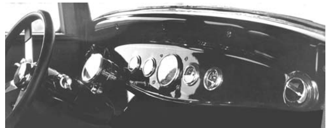
49260-VFI (below) 1928-32 Ford fiberglass dash with built-in louvers at each end for a super smooth look. Fits coupes and sedans.
