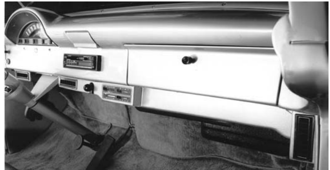
Underdash panel with louvers package shown is available with or without control panel installed.
