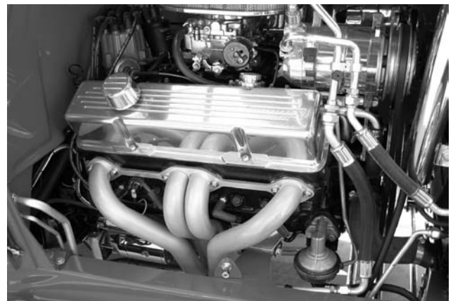
Neatly routed hardlines give your engine compartment a professional look.
