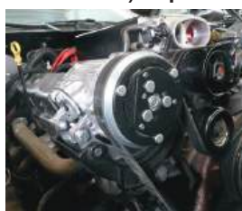
151585 Serpentine R4 to 7B10 adapter bracket (fits 1988-92 GM "F" and "B" body, and 1988-89 GM and Chevy trucks).
