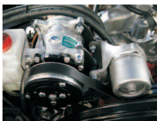
141805 Sanden / R4 multi-groove conversion bracket
