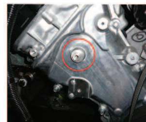
Revision 2-Timing Cover with different boss on cover
