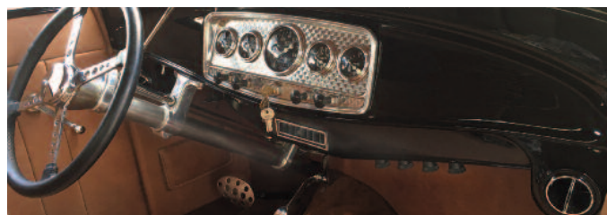
491200-RUA Gen II 4-Knob Controls (Mounted behind dash) 49053-VUL ProLine Louvers
