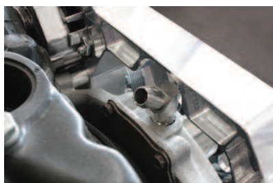
OEM-Style Water Pump Bypass Design
