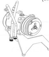
1935 Models up with top mount steel compressor bracket
