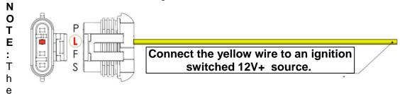
ellow turn-on wire from the supplied alternator pigtail can be extended with any 12 to 16 gauge wire.
