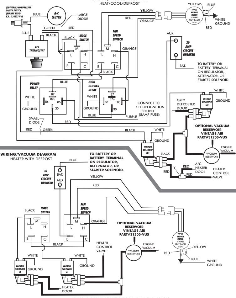
901428 REV B 10/5/12, INST 28" PUSH-PULL CABLE w/ ROTARY SWITCH PG 2 OF 3
