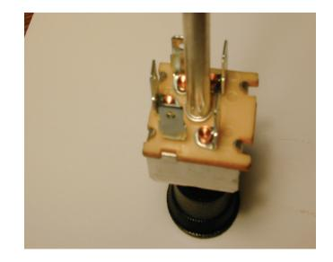
WIRE THE SWITCH BY FOLLOWING THE WIRING DIAGRAM SUPPLIED WITH YOUR A/C SYSTEM INSTRUCTIONS. THE SWITCH HAS 5 SPADES ON THE BACK. THE SPADE MARKED (C) PROVIDES THE SAME FUNCTION AS A SPADE MARKED (AC) ON A DIFFERENT SWITCH.
