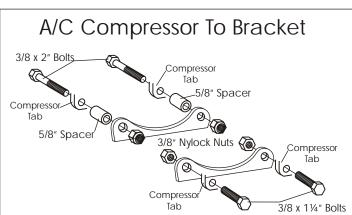
This bracket is designed for the Sanden 508 compressors, and a standard case GM alternator equipped with a two groove pulley. The two groove alternator pulley came standard on all factory air Rivieras, and can also be found in the aftermarket.
