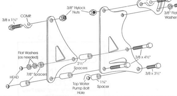
We use a belt length of 591/2-601/2" with this mount on installations in our shop. However; this can vary with the diameter of your pulleys.
