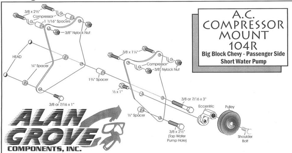
NOTE: Some heads have 3/8" bolt holes and some have 7/16". This kit includes both sizes of bolts for these holes.
