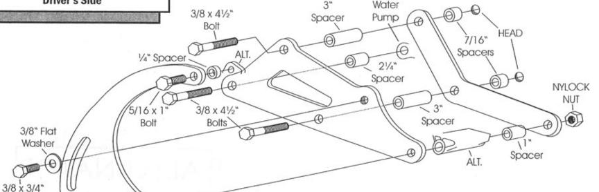
The alternator belt will run in the second grooves from the front of the crank and water pump pulleys originally used for the factory compressor. It was designed to be used with our Passenger Side Compressor Mount.
