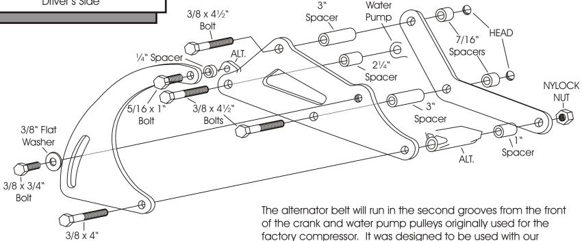
It can be used with single groove crank and water pump pulleys by using a double groove alternator pulley and running the belt in the outer groove.
