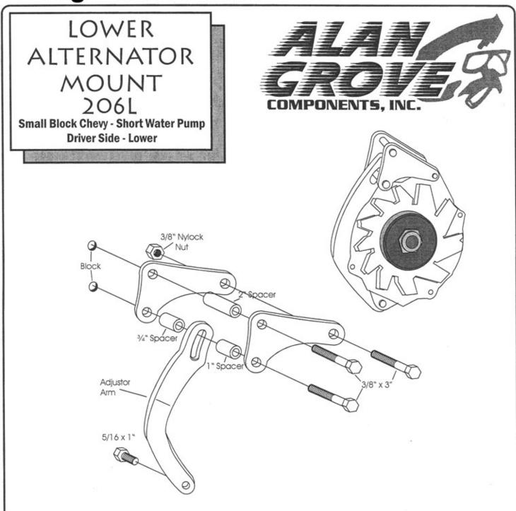
(We use a belt length of  $42\frac{1}{2}$  to  $43\frac{1}{2}$ " with this mount on installations in our shop. However; this can vary with the diameter of your pulleys.)
