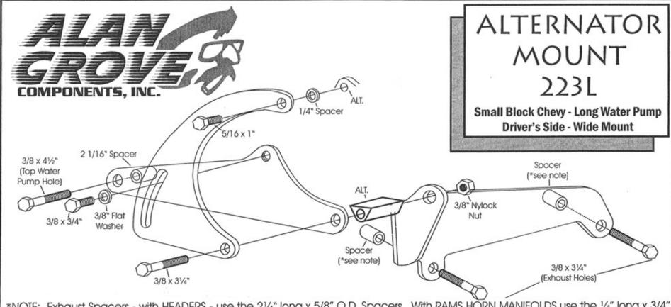
\*NOTE: Exhaust Spacers - with HEADERS - use the 21/4" long x 5/8" O.D. Spacers. With RAMS HORN MANIFOLDS use the 1/4" long x 3/4" O.D. Spacer at rear hole of bracket and a 1 1/16" long x 3/4" O.D. spacer at front hole of bracket. With the later DROP-TYPE MANIFOLDS use the 1 1/16" long x 3/4" O.D. Spacers at both bracket holes. As with any mount system, assemble all of the brackets to engine BEFORE tightening the bolts.
