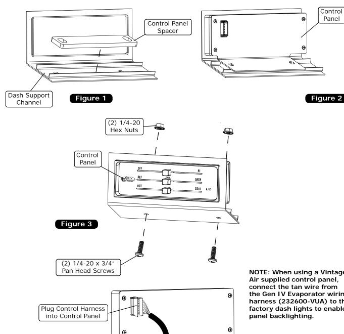
NOTE: When using a Vintage Air supplied control panel, connect the tan wire from the Gen IV Evaporator wiring harness (232600-VUA) to the factory dash lights to enable
