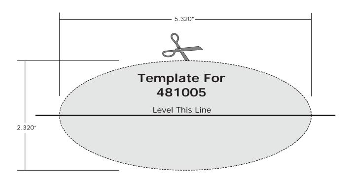
NOTE: Ensure that the template measures to dimensions noted above prior to cutting dash.
