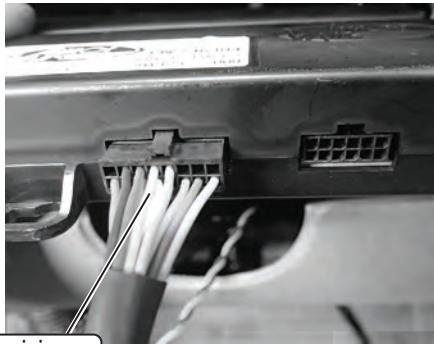
Plug main wiring harness connector into ECU module
