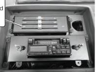
Connect control panel harness plug into ECU
