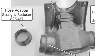
Use OEM duct hose on this side and route to driver-side louver
