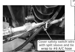
Connect compressor bullet connector to compressor lead
