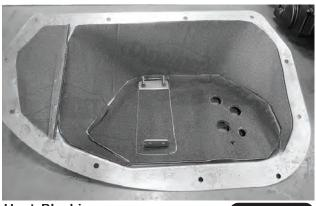
Heat-Blocking Insulation Installed
