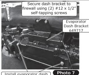
Install evaporator dash bracket using (2) 1/4-20 x 1" serrated flange bolts
