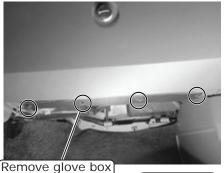
door by removing (4) screws
