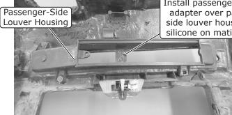
Install passenger-side hose adapter over passengerside louver housing, using silicone on mating surface
