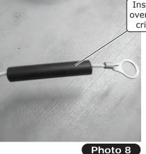
Install supplied heat shrink over white ground wires and crimp on supplied eyelets
