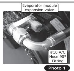
Evaporator module expansion valve
