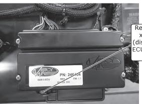
Remove (2) #10 x 5/8" screws (discard) securing ECU to evaporator module
