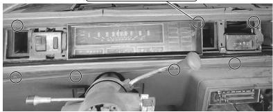
Disconnect speedometer and remove gauges by removing (4) screws
