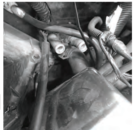
Heater Hoses Removed
