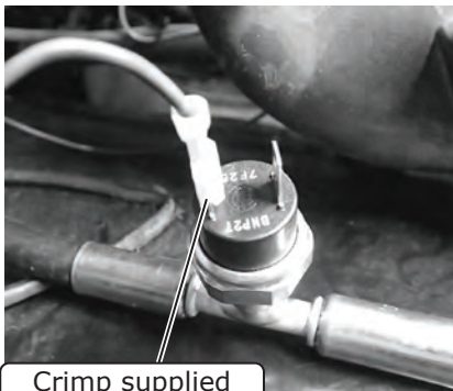
Crimp supplied female spade terminal connector onto blue wire and install it onto binary switch
