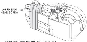
**SECURE USING (2) #6 x 3/8 PH** PAN HEAD SCREWS AS SHOWN
