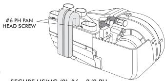
SECURE USING (2) #6 x 3/8 PH PAN HEAD SCREWS AS SHOWN
