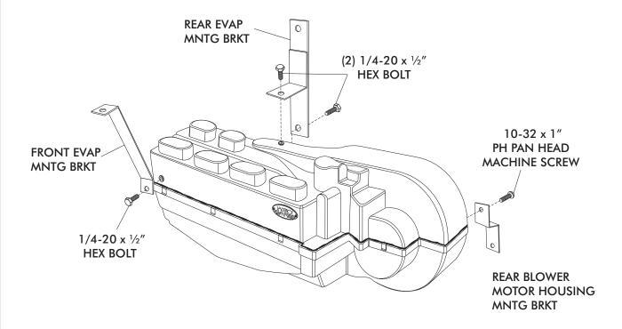
REMOVE THE (3)  $1/4-20 \times 1/2$ " COARSE HEX BOLTS FROM THE SUB CASE AND INSTALL FRONT AND REAR EVAPORATOR MOUNTING BRACKETS AS SHOWN.
