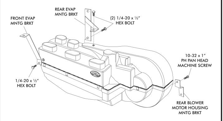
REMOVE THE (3)  $1/4-20 \times 1/2$ " COARSE HEX BOLTS FROM THE SUB CASE AND INSTALL FRONT AND REAR EVAPORATOR MOUNTING BRACKETS AS SHOWN.
