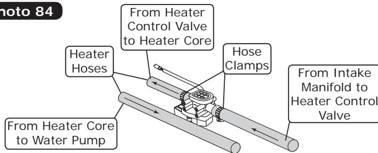
**NOTE: Flow Direction Follows Molded Arrow on Valve.**
