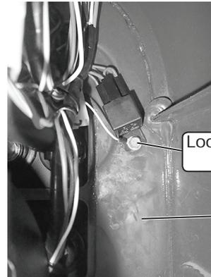
Loosen Relay Bolt
