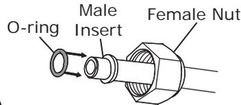
For a proper seal of fittings: Install supplied O-rings as shown, and lubricate with supplied oil.
