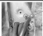
Secure firewall using (5) 10-24 nuts with star washers
