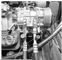
Install straight fitting of #8 A/C hose to discharge port on compressor
